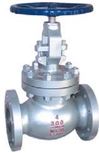
FIG. 276-CS-300 Class 300, Flanged ends, bolted bonnet, WCB body & bonnet, 13Cr/HF trim.
